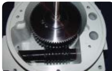
Self Locking worm and gear transmission system
